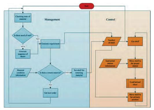
Fig. 3. Simplified diagram of the depot operation
